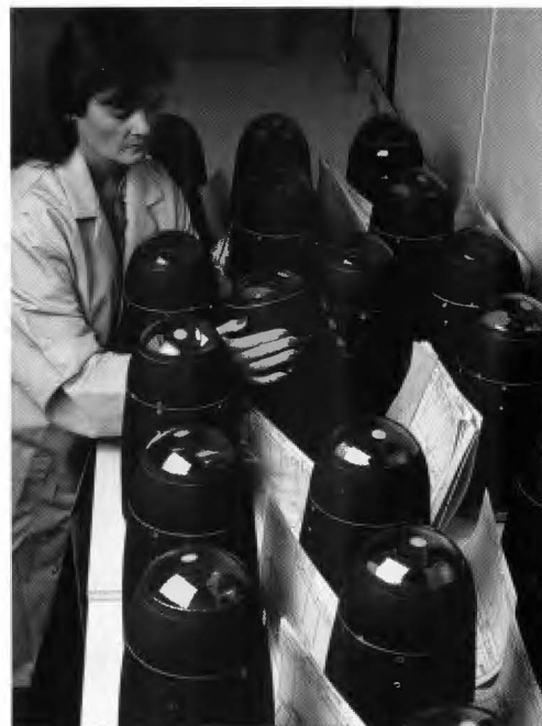
Gail Bates inspects laser seekers developed by Martin Marietta for the Army's Hellfire anti-armor missiles. The Corporation also co-produces the air-to-surface missile.
