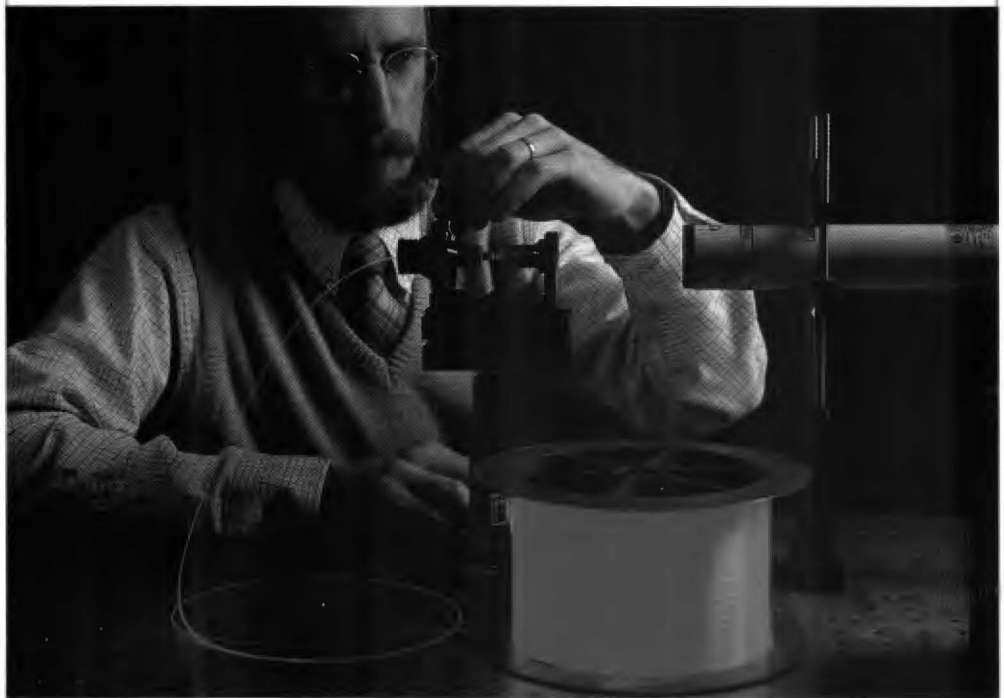
Laser light illuminates a 500-meter spool of optical fiber, which Baltimore Aerospace engineer Russell May aligns in an experiment to develop secure communications.
