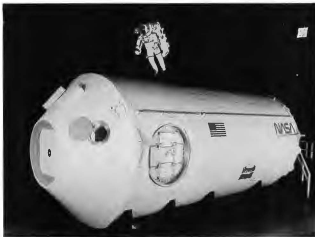
Space Station common module mockup
