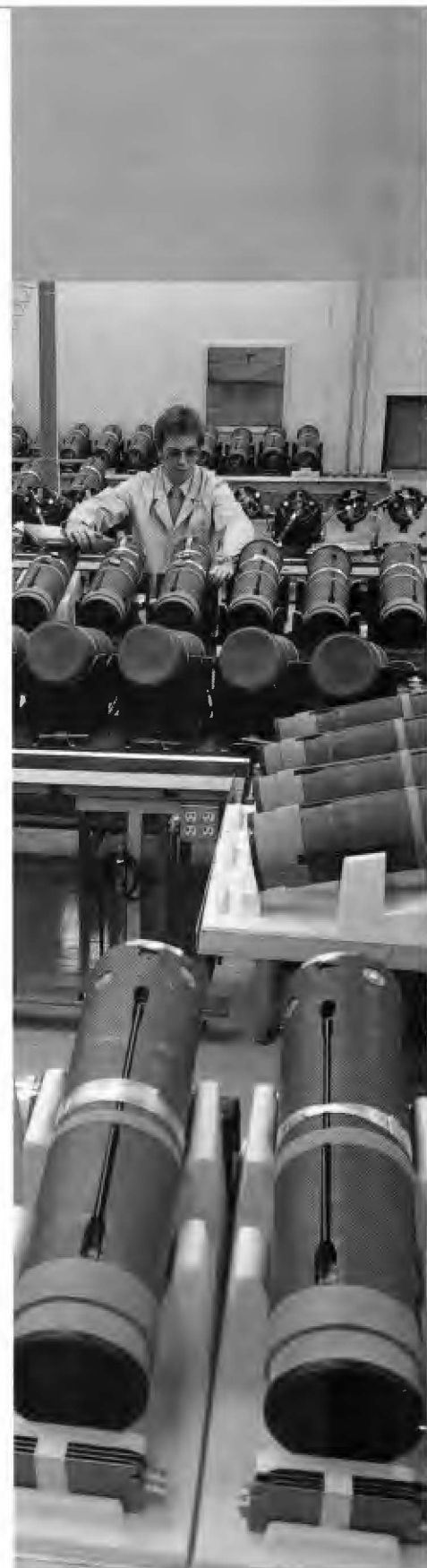
Robert Evick inspects control sections for the Copperhead laser-guided projectile at Ocala, Florida, before the highly accurate artillery shells are delivered to the Army.
