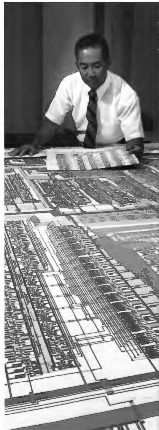
Orlando design engineer Robert Yokomoto examines the diagram for a very large scale integrated circuit that will be reduced to a single chip layer with circuit lines one-fiftieth the thickness of a human hair.
