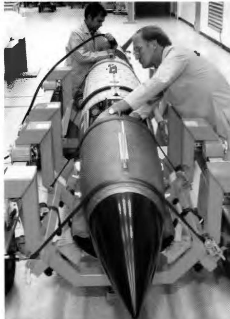
Ernest Buckley (left) and Michael Neener perform engineering tests on a Mach 2.5, low-altitude target drone under development for Navy missile defense training and evaluation.
