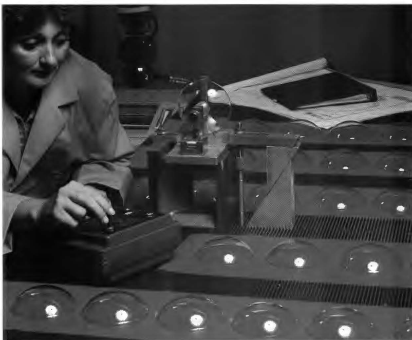
Orlando's Roseanne Freeman precisely measures the curvature of a plastic dome for a laser guidance system.
