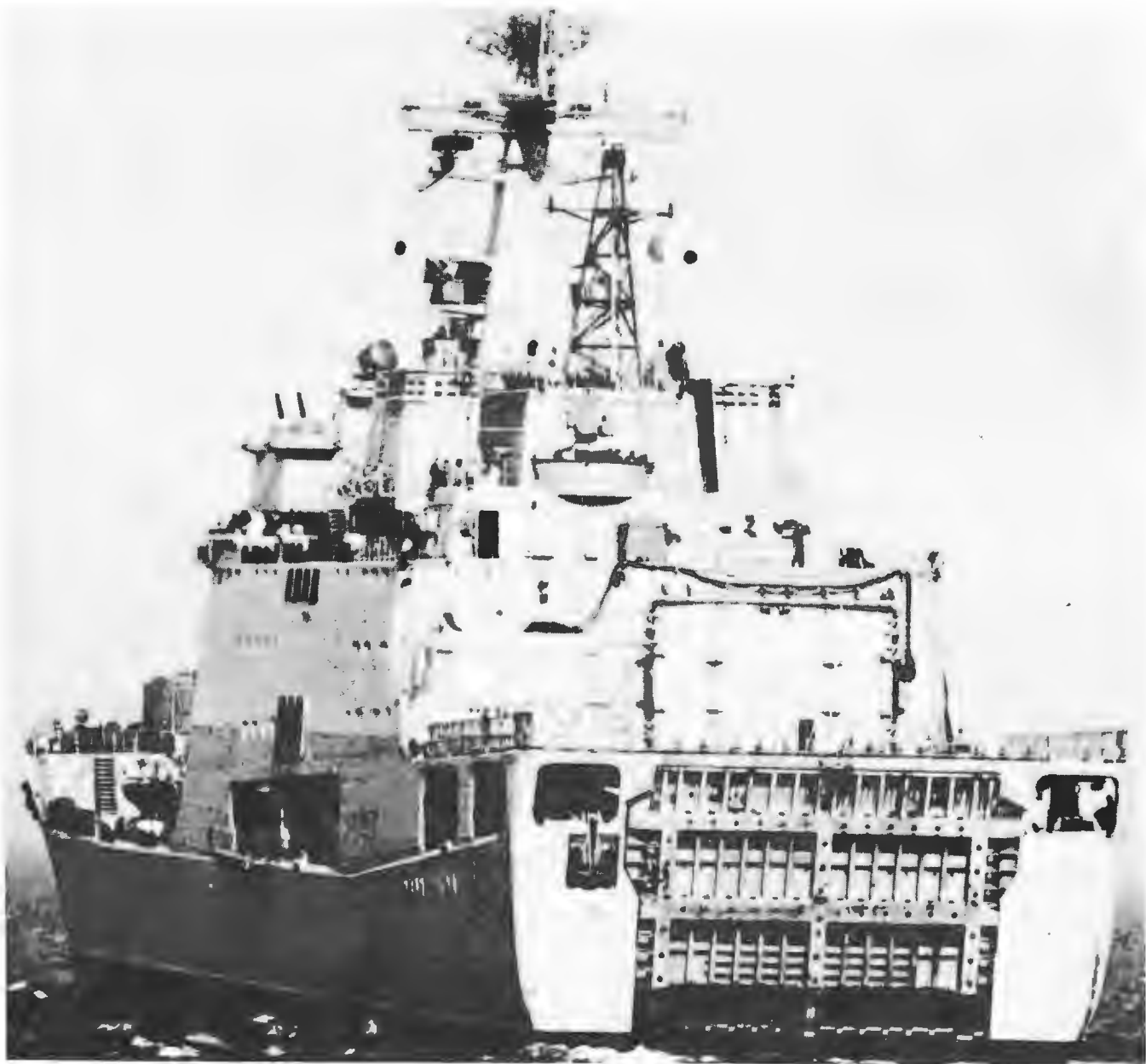
The 13,000-ton amphibious assault transport dock IVAN ROGOV entered service in 1978, the largest amphibious ship in the Soviet Navy. IVAN ROGOV has two helicopter decks and helicopter hangers, and a floodable welldeck, behind the large stern gate, which can carry three air-cushion landing craft. Judging by IVAN ROGOV's characteristics, the amphibious ship can carry a Soviet Naval Infantry Battalion—550 men—30 armored personnel carriers and ten tanks, enhancing the USSR's capability to project naval and military power at great distances from the Soviet homeland.
