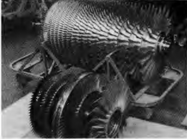
The Soviet R-11-300 rotor assembly (left photo, foreground) performs essentially the same work as that of the US J-79 (in back). The right photo shows the R-11-300 compressor components.
