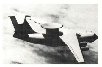
The new II-76/MAINSTAY aircraft is illustrated as configured for its Airborne Warning and Control Systems mission.
