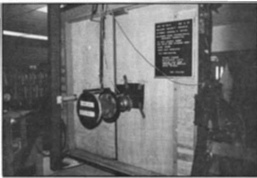
Test Fixture, Developed by CCTRF to Simulate Human Threats to Door Systems
