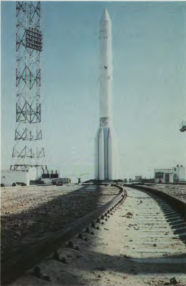
The Soviets first launched the SL-12 vehicle, the "Proton" (similar to the US Titan), in 1967. This four-stage space booster is used to launch communication and navigation satellites, interplanetary probes, and, in the SL-13 three-stage version, the SALYUT and MIR space stations. The Soviets are now advertising the Proton for worldwide launch services at half the cost competitors are asking.
