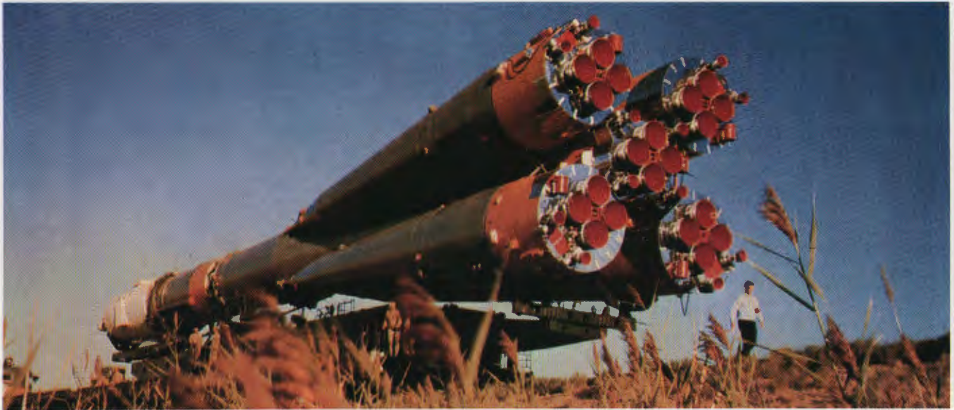
An example of how the Soviets transport a fully integrated launch vehicle is shown above. The SL-4, which is used to place cosmonauts, resupply vehicles in support of the MIR space station, and many other payloads into orbit, is transported to the pad by rail and then erected for launch.
