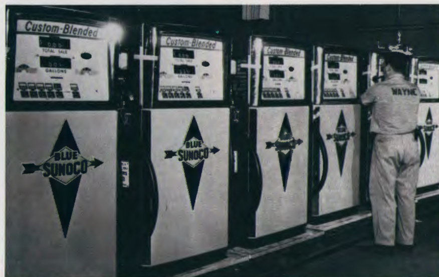
Custom blending was a unique response to expanding engine octane requirements of 1950s.
