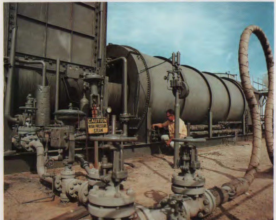
Equipment required to increase recovery by injecting steam into one of Sun's older fields in California underlines the need for sufficient incentives to make such investments attractive.
