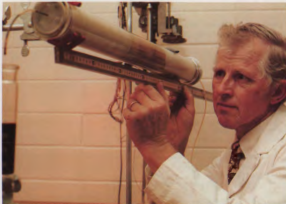
Core samples, like the one analyzed by Dr. Earl Malmberg of Sun's Richardson lab, give details of rock composition to help determine which method of enhanced recovery will work best.
