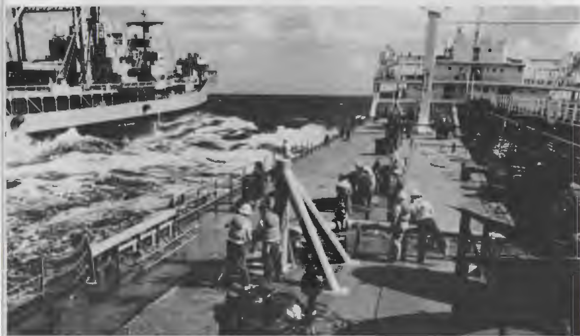
The 1972 test series in which the merchant tanker Erna Elizabeth was used to refuel Navy combatant ships at sea proved the feasibility of the concept, but a follow-on program was never authorized.
