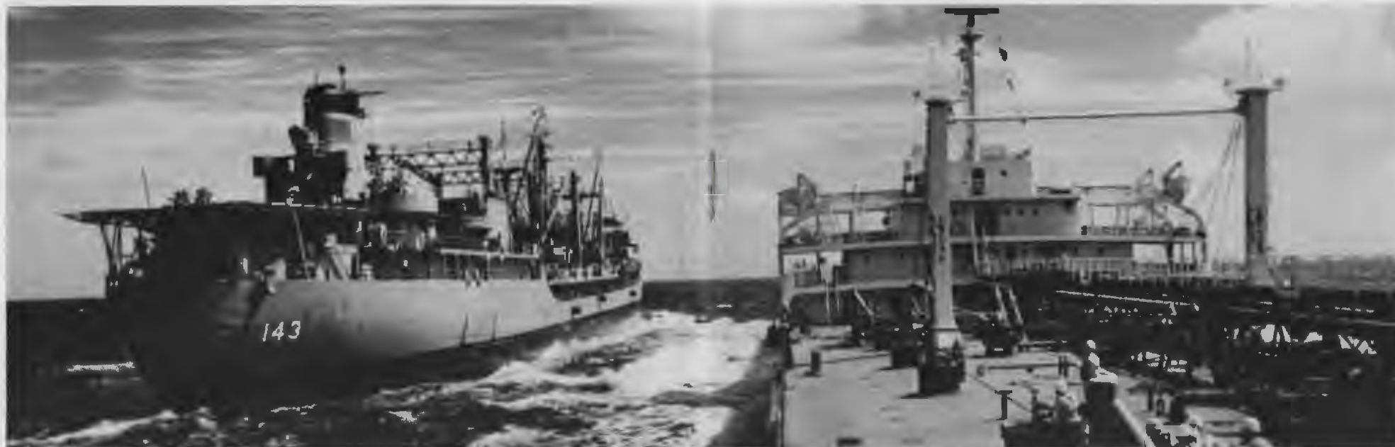
The 1972 test series in which the merchant tanker Erna Elizabeth was used to refuel Navy combatant ships at sea proved the feasibility of the concept, but a follow-on program was never authorized.
