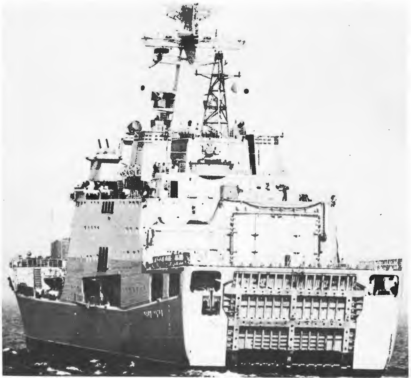
The 13,000-ton amphibious assault transport dock IVAN ROGOV entered service in 1978, the largest amphibious ship in the Soviet Navy. IVAN ROGOV has two helicopter decks and helicopter hangers, and a floodable welldeck, behind the large stern gate, which can carry three air-cushion landing craft. Judging by IVAN ROGOV's characteristics, the amphibious ship can carry a Soviet Naval Infantry Battalion—550 men—30 armored personnel carriers and ten tanks, enhancing the USSR's capability to project naval and military power at great distances from the Soviet homeland.
