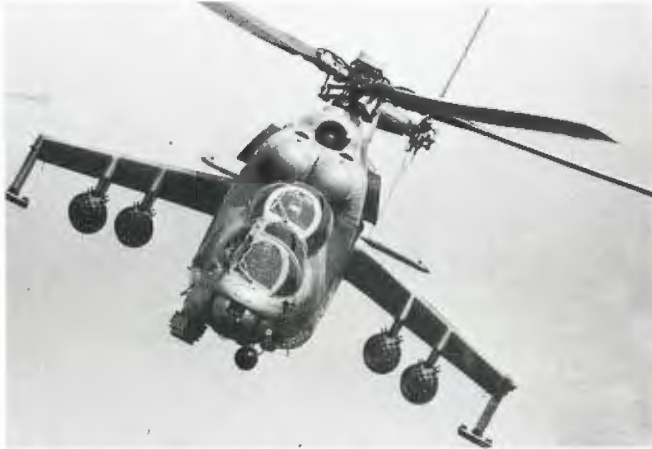
Mi-24/HIND E with Tube-Launched Anti-Tank Guided Missiles
