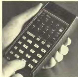
The "electronic slide rule" was born in January, 1972, with introduction of the HP-35 scientific calculator. A large family of small Hewlett-Packard calculators followed, including the world's first programmable hand-held calculator.
