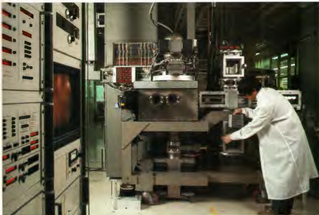
ELECTRON-BEAM SYSTEM DEVELOPED BY HP LABORATORIES FOR INTEGRATED CIRCUIT PRODUCTION.
