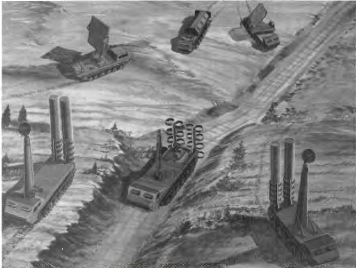
The surface-to-air missiles of the SA-X-12 air defense system are designed to counter high performance aircraft and will also have a capability against tactical ballistic missiles.
